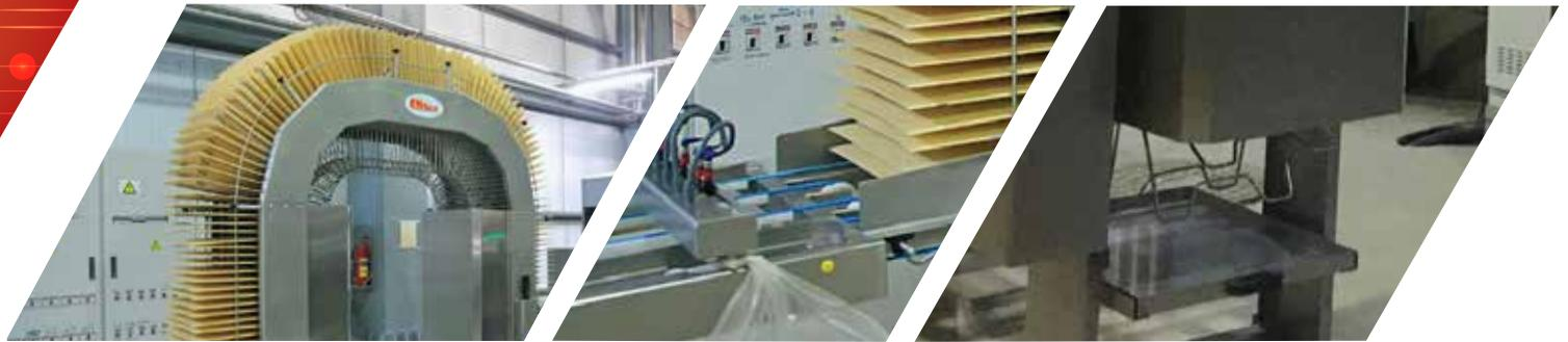
Designed to cool the wafer sheets to room temperature. Synchronize work with the Wafer Baking Oven. Food Safe materials are used to produce. Automatically discharge the broken wafer sheets
