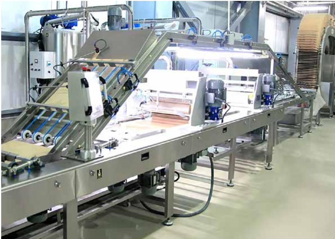
Designed to spread cream to wafer sheets. Wafer sheets move separately from up and bottom side to increase capacity. Wafer Cream Spreading System can produce 2-5 lines of cream. Height of the cream line can be set. After spreading cream, wafer block is adjusted from all side and send to Wafer Block Cooling System.
