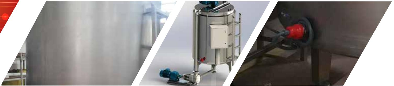
Designed to prepare marshmallow syrup before aeromix. Marshmallow Preparation System includes three different tank to boil, rest and use tanks. All parts that touch the product made by Stainless Steel AISI 304. Temperature of the marshmallow syrup is regulated by jacket system. There are filters between tanks and marshmallow syrup is transferred by pumps. To transfer the marshmallow syrup to aeromix special pump is used to keep pressure of syrup stable.
