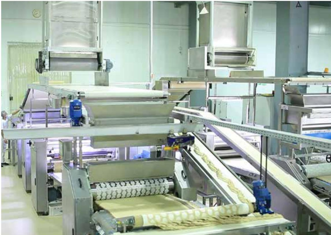
Designed to feed and form the hard and soft biscuit. Used to shape and cut the hard dough and shape the soft dough with feeding system. Rotative machine can be controlled by its own control panel and can be synchronized with dough feeding and lamination group. Rotative machine includes the returning belts to use remaining dough sheet after cutting.
