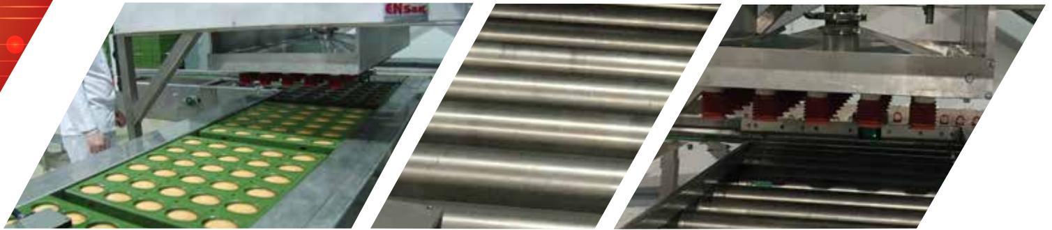
Designed to discharge the cake pans. Cake Depanning system differs according to product range. Vacuum system takes the cakes from pan and put them to the transfer conveyour. Allows to take different kind of cake products from pans. Type of Cake Depanning System differs according to production area and products that are produced in the production line.
