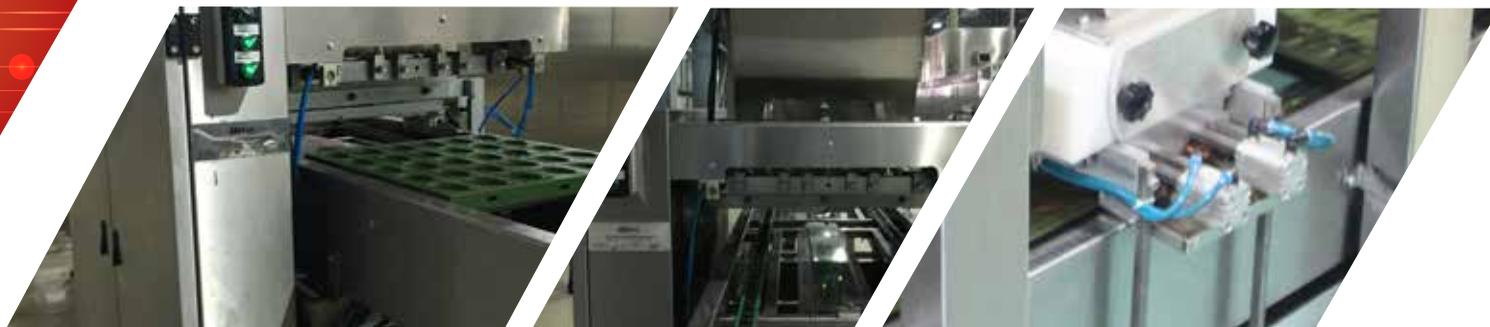
Designed to place liquid cake dough to the center of pan cells. Servo-Motors are used to control the weight of the dough. Cake Dough Depositor allows to produce different kind of products. Electronic sensors control the movement of the depositor. Easy to clean. Each nozzle can put between 20-75 gr of cake dough to each pan cells. Weight control is sensitive because of the Servo- Motors and easy to adjust the weight of the dough.
