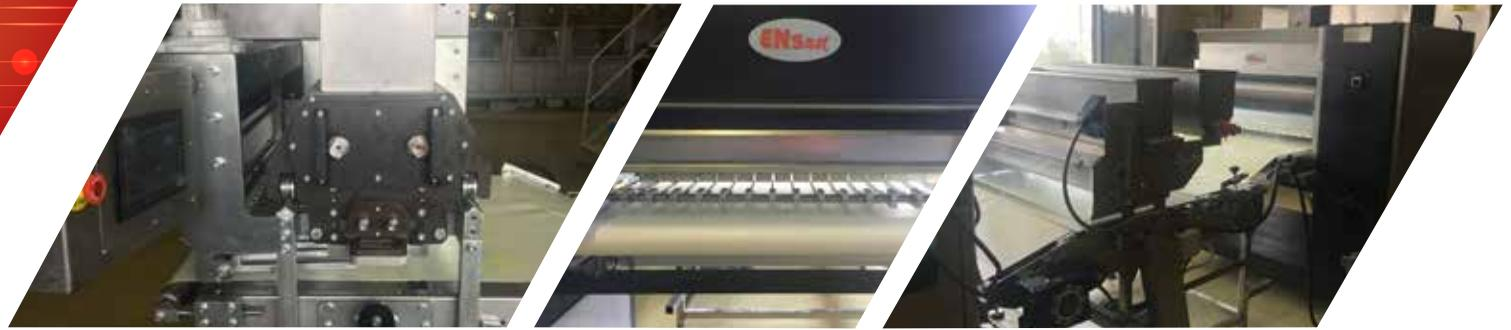
Designed to form cookie doughs in shape of heart, rectangle, triangle etc. Servo motor controlled dough feeding gives user sensitive weigh control of the dough. Sesame, Salt spriller system can be adaptable.
